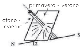
Fig. 20: Equatorial clock in used in northern hemisphere.
