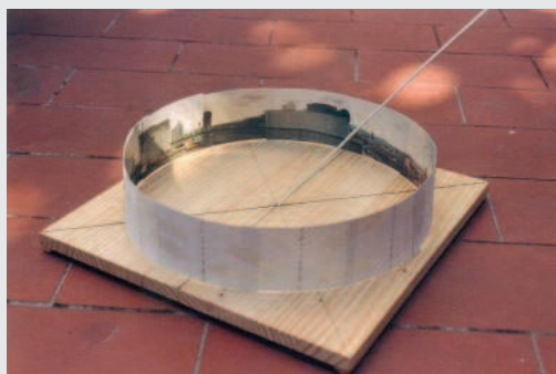
Fig. 10: Model with horizon ring and polar axis.
